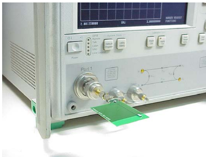
Testing Instrument: Anritsu 37369C VNA(Vector Network Analyzer)
