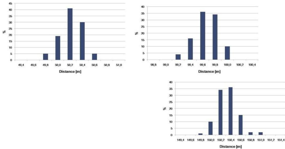
**Figure 5 Ranging Accuracy** - Ranging Accuracy is characterized by offset and spread. The actual distances are 50, 100, and 150m respectively
