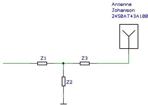
**Figure 2-3** Sample matching network of chip antenna
