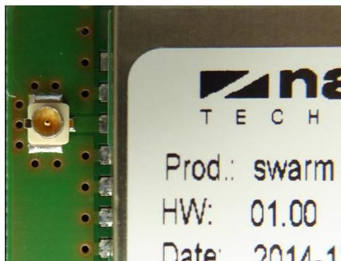
**Figure 2-4** U.FL connector on a PCB
