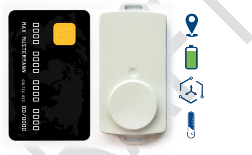
Figure 2 assetTAG-c (94 mm x 43 mm x 14 mm)
