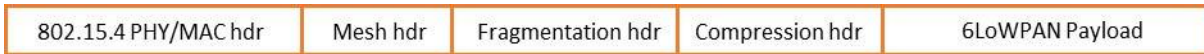
Figure 8. 6LoWPAN Packet Containing Mesh Header, a Fragmentation Header, and a Compression Header
